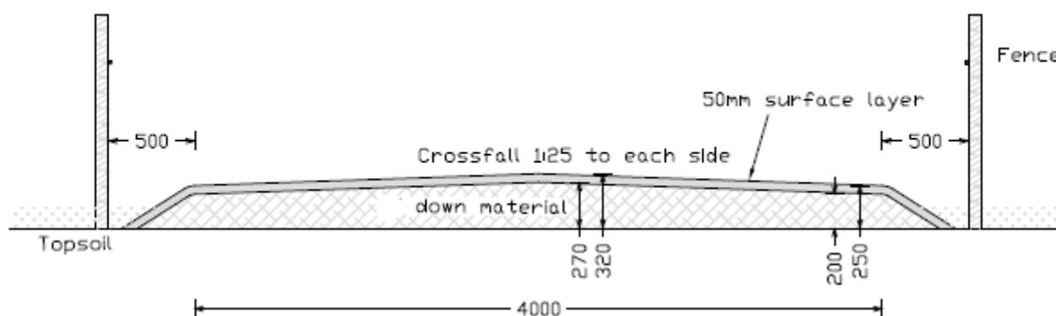
**Figure 3** New Farm Roadway with Camber from the centre (not applicable for compliance with Regulations - S.I. No. 605 of 2017)
