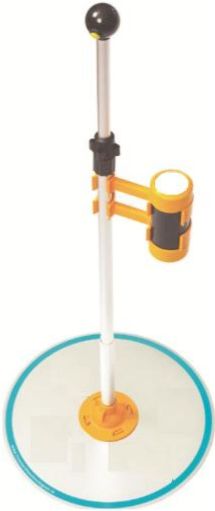
**Figure 1:** Example of a rising plate meter
