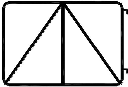
**Figure E1.3 Construction of Steel Gates (Pattern for Timber Gates)**
