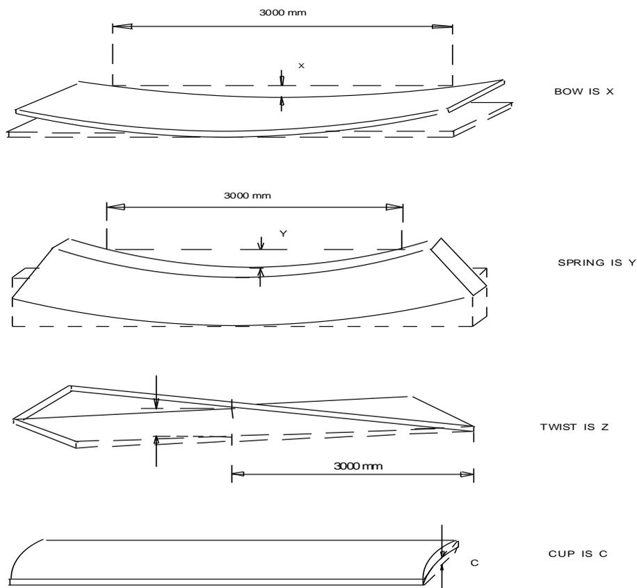
Figure 1 — Timber post and rail horse/stud fencing - measurement of bow, spring, twist and cup
