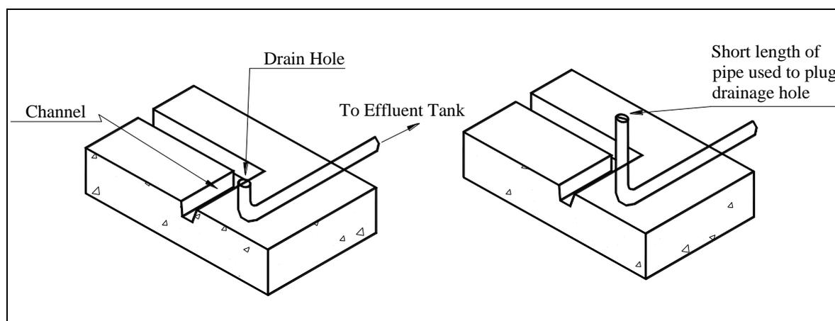
**Figure 3** Diversion Trap for Cleanwater Run-off
