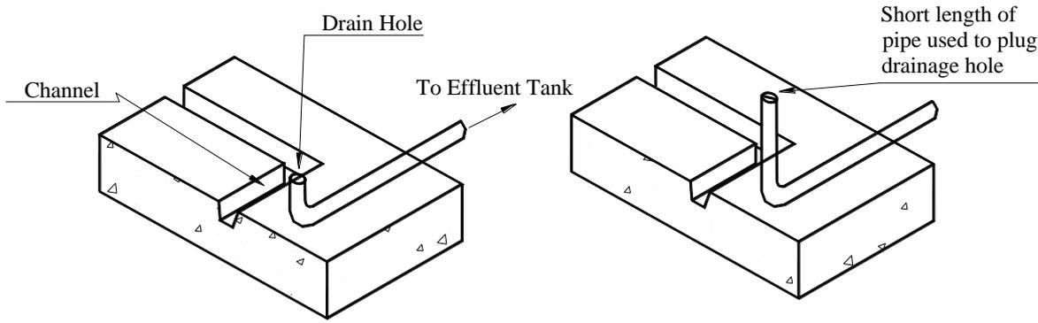
**Figure 2**      **Diversion Trap for Cleanwater Run-off from Base**
