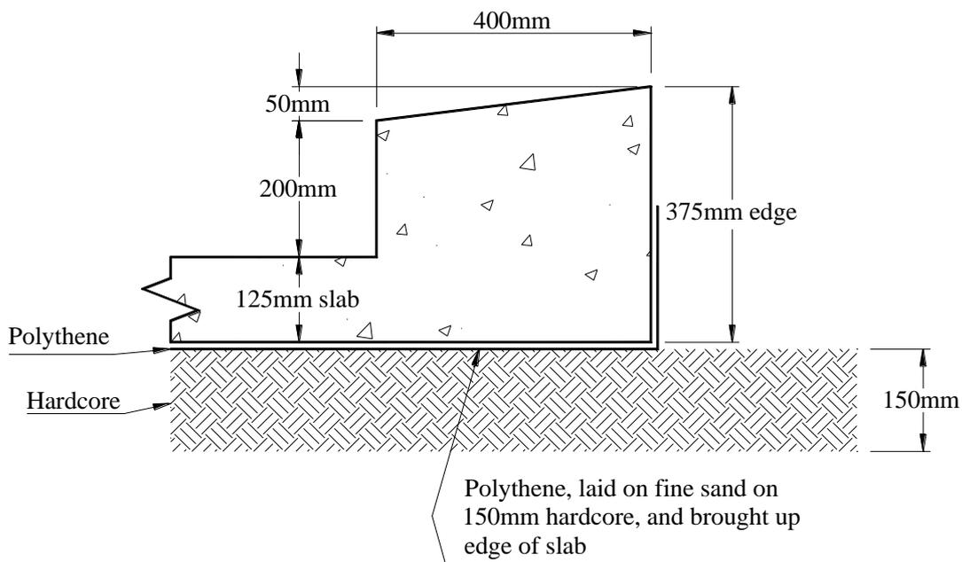
**Figure 4 Side-Edge / Back-Edge (Kerb-Type)**
