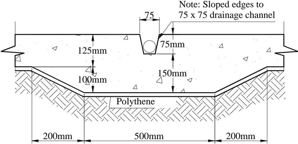
**Figure 7 Cross-Channel / Alternative Front-Channel**
