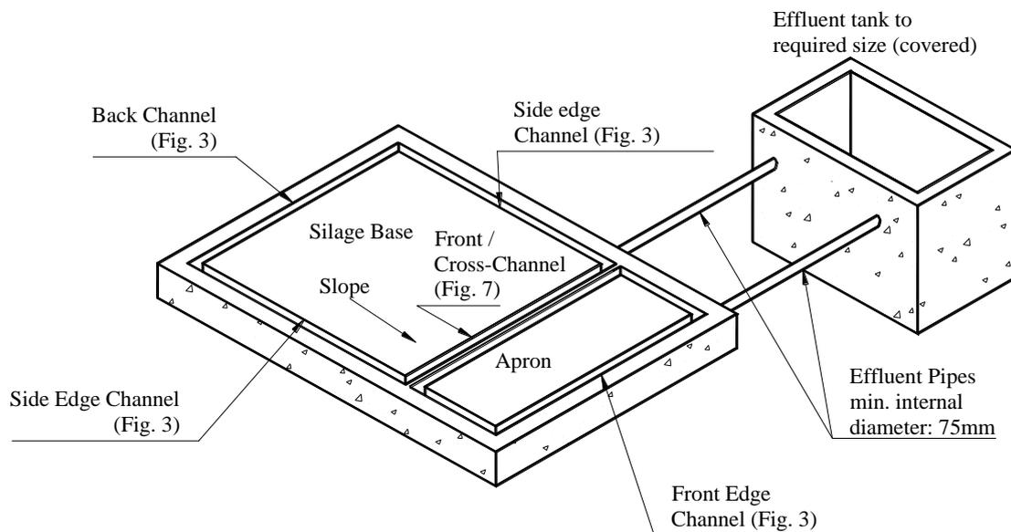
**Figure 1 Construction of Silage Base and Tank**
