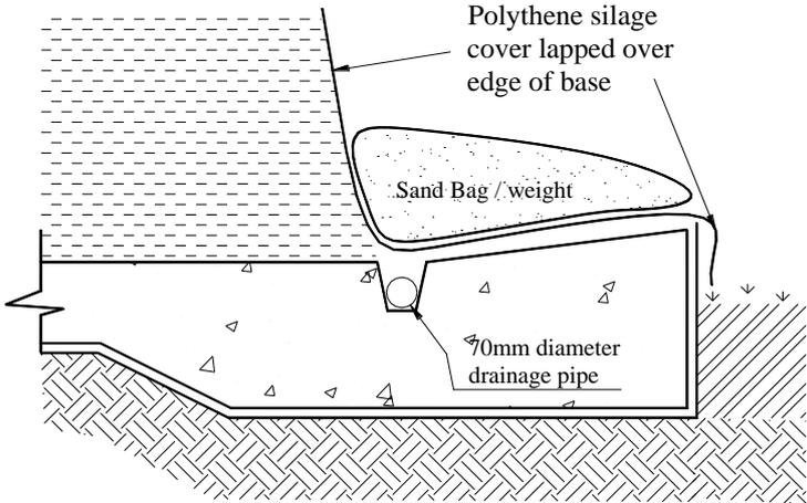
**Figure 5 Side-Channel in Use**
