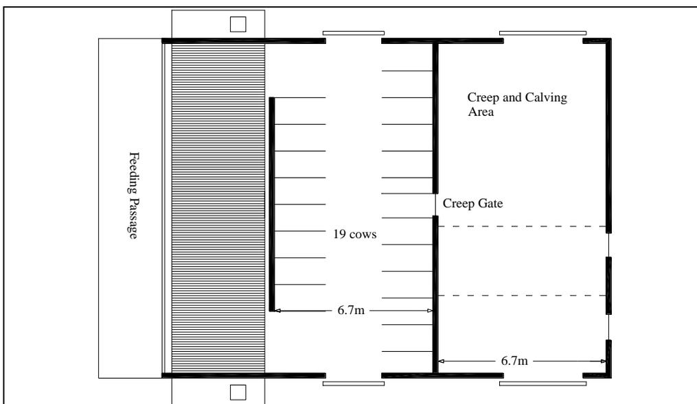
**Figure 4 Adapted Existing Housing / Cubicle - Easy Feed**
