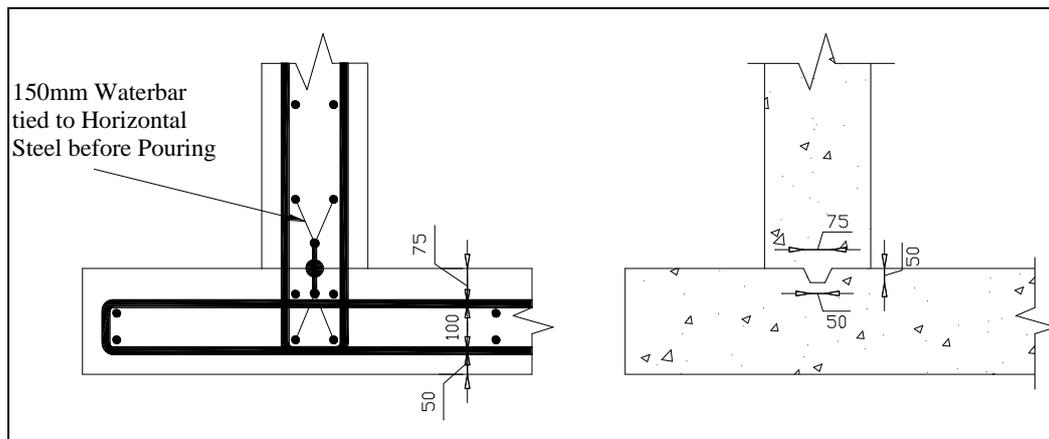
**Figure 12 Wall-Floor Joints**
