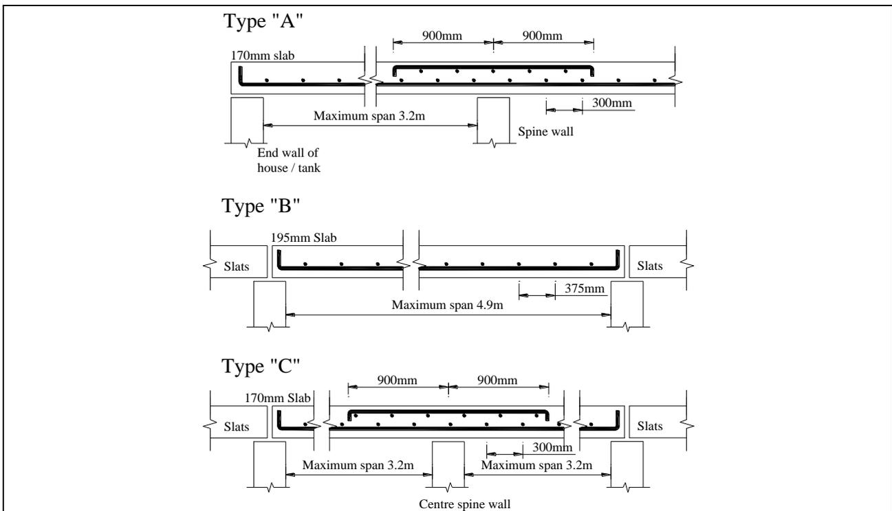
**Figure 18** Suspended Slabs: Steel Details
