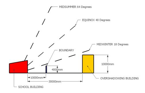
The diagram above illustrates the elevation of the sun throughout the year. The direction of the sun is illustrated from a due south position at noon.
