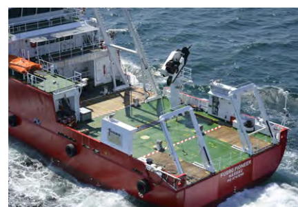
Limited draft makes it specifically suitable for survey nearshore.
