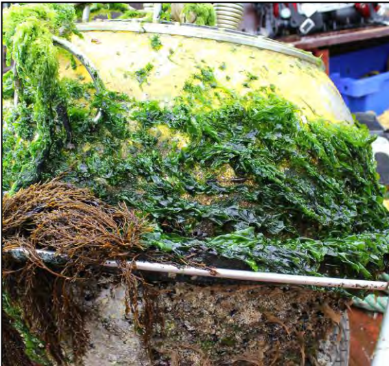
Fouling after fourteen weeks at sea.
