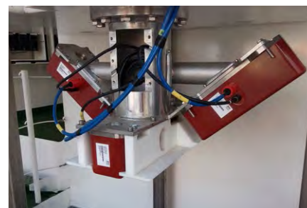
State of the Art Kongsberg Dual Head Dual Ping Multibeam in retractable moonpool system.
