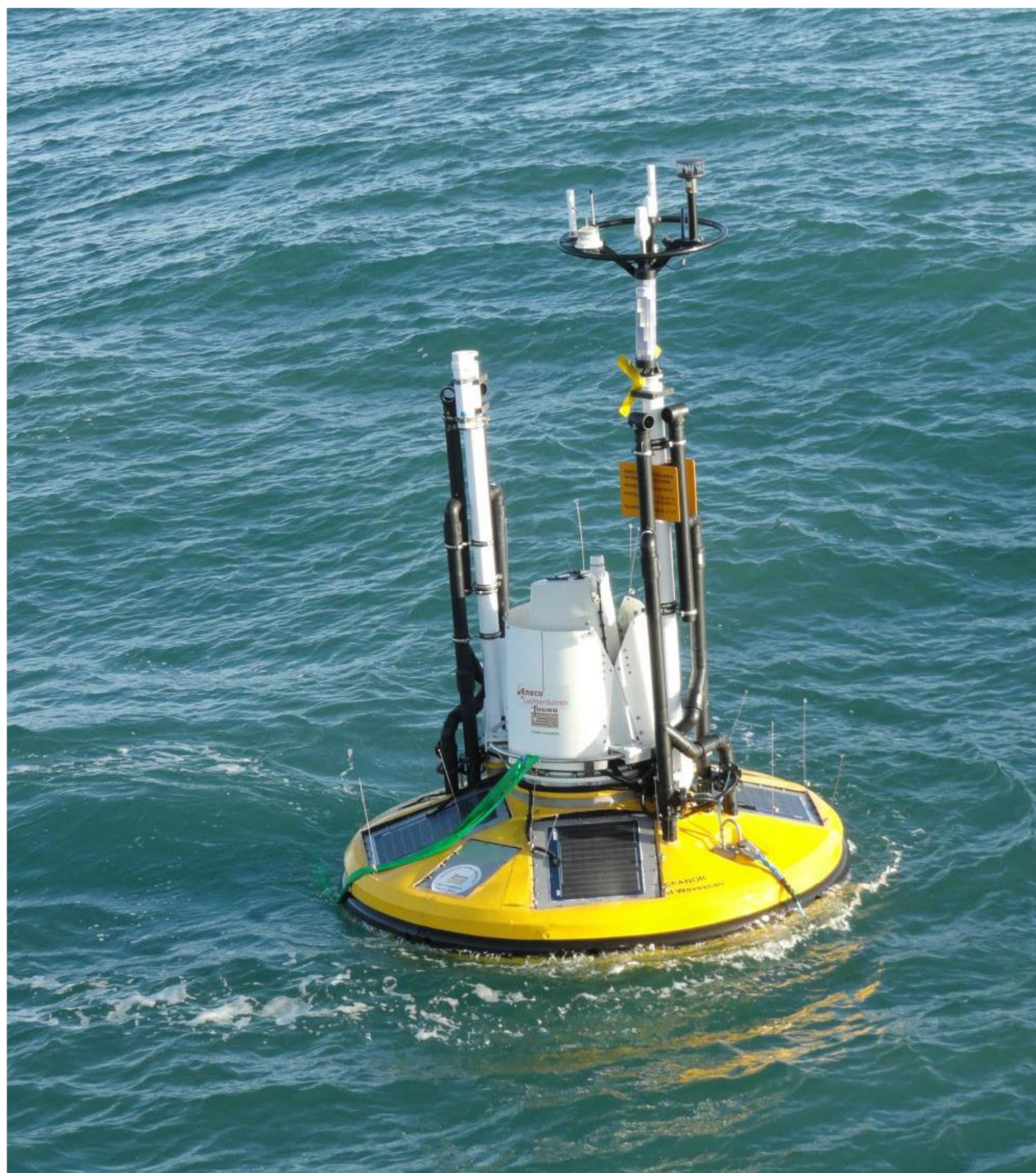
Photo 1 - Wind LiDAR Buoy
