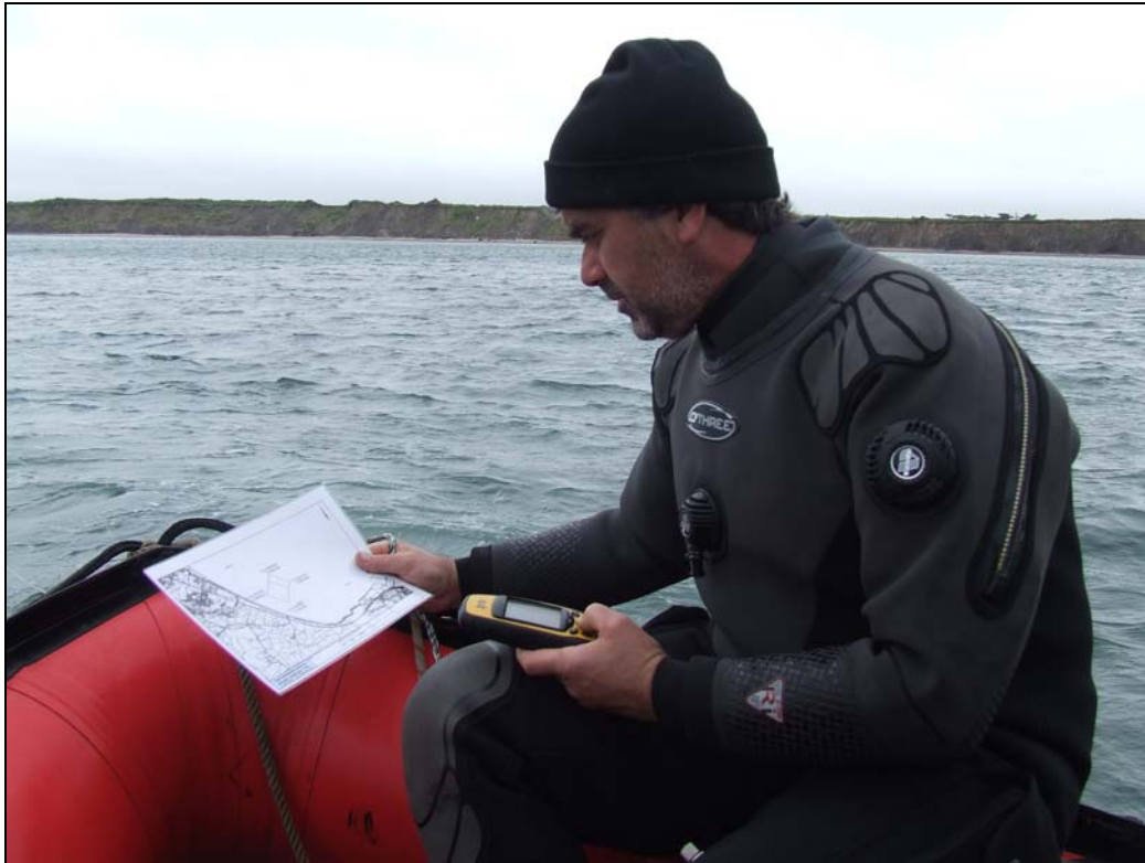
Plate 3: Working shot of diver establishing coordinates for the dropping of surface marker buoys at the four corners of the survey area.
