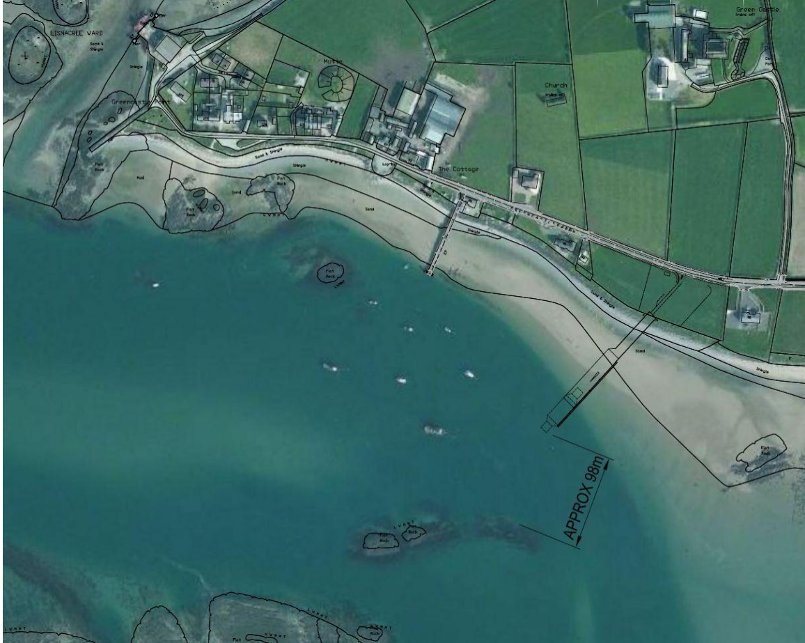
Annex 1: Proposed Pier with Ferry outline - Satellite Image showing Distance from Rocks.
