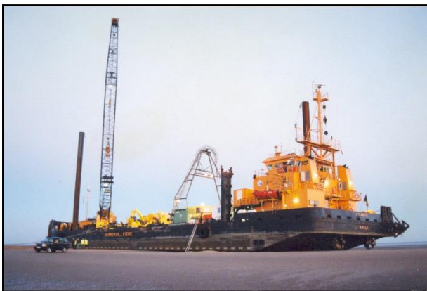
Figure 3. Typical Shallow Draft Lay Vessel
