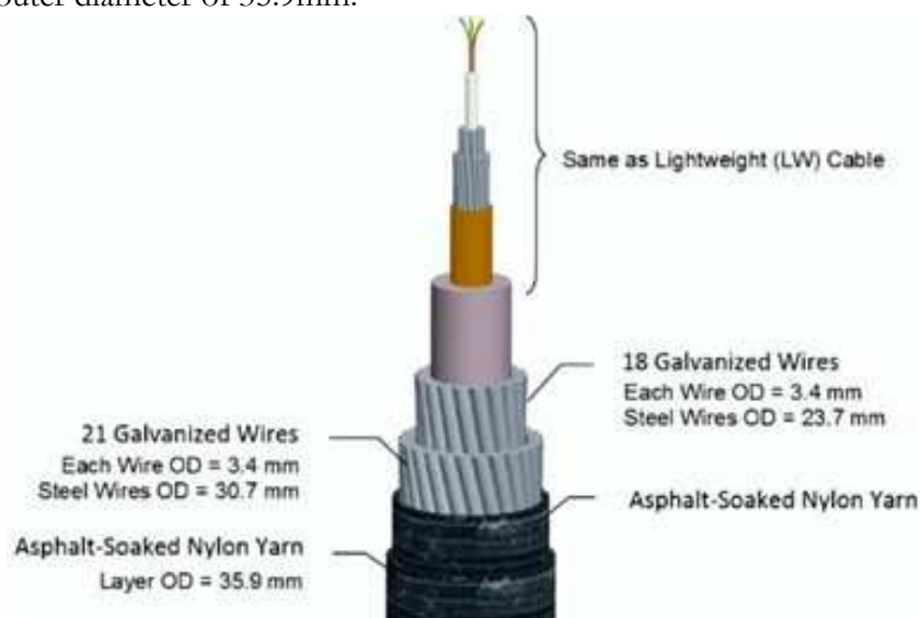
Figure 4. Cut-Away Section of Double Armour Cable
