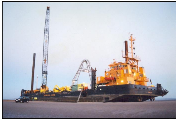
Figure 26. Typical Shallow Draft Cable Lay Vessel.
