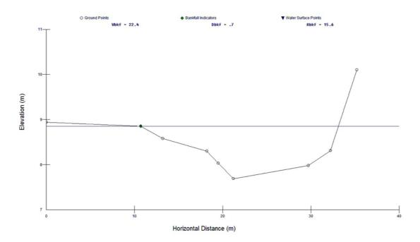
Figure 5.5. Channel dimensions at location of cross-section levelling.
