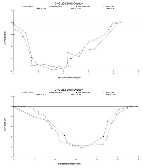
Figure 3.6. Comparison of cross-sections from 1999 (pre-maintenance – green line) and 2018 (black line) for chainage 228 (top) and 232 (bottom). See photographs below.
