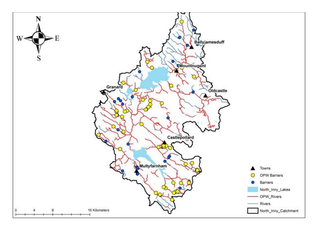
Figure 1.14. Distribution of barriers identified around the Northern Inny Catchment in 2018 (Yellow Circles are OPW registered Structures; Blue Circles are other structures posing problems).
