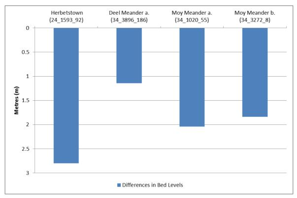
Figure 5.8. Stage or vertical height (m) differences between existing river bed level adjacent to meanders and bed level in meander. 0 on x axis is the current bed levels of each meander.
