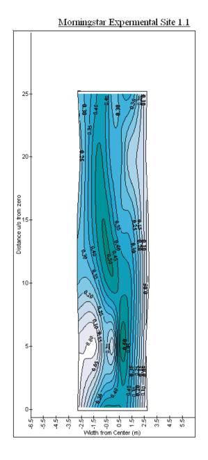
Figure 3. Depth contour plot for site 3 on the Morningstar experimental site in the Maigue Catchment, August 2008
