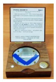
The densiometer consists of a curved concave reflecting mirror and has 37 grid intersection forming 24 squares. Only 17 of the line intersects are used as recording points by taping a right angle on the mirror surface as shown in Figure 4. Canopy density/closure is measured at 4 or 8 points in the stream depending on width.
