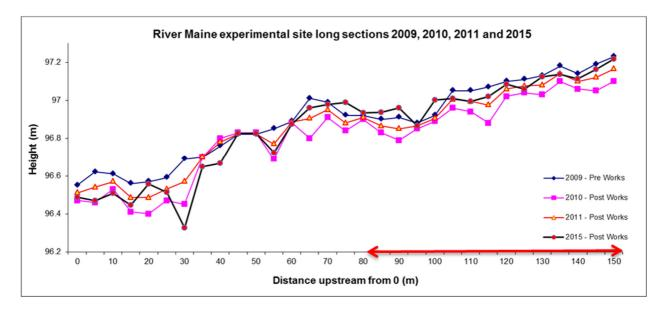
Figure 4.10. River Maine experimental site long sections pre (2009) and post works in 2010, 2011, 2015 (arrow indicates location of depth contour plot in Figure 4.11).
