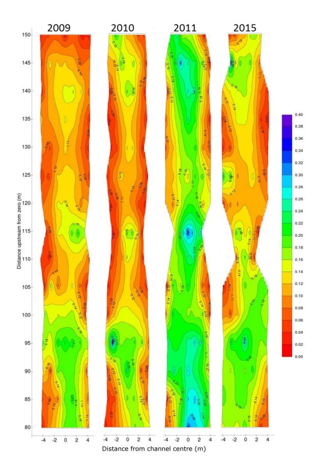
Figure 4.11. Depth contours of a section of the River Maine experimental site: pre works (2009) and post works (2010, 2011 and 2015).
