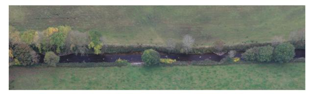
Figure 4.8. Aerial view of the River Maine experimental post works October 2009 (note alternating deflectors and random boulders).
