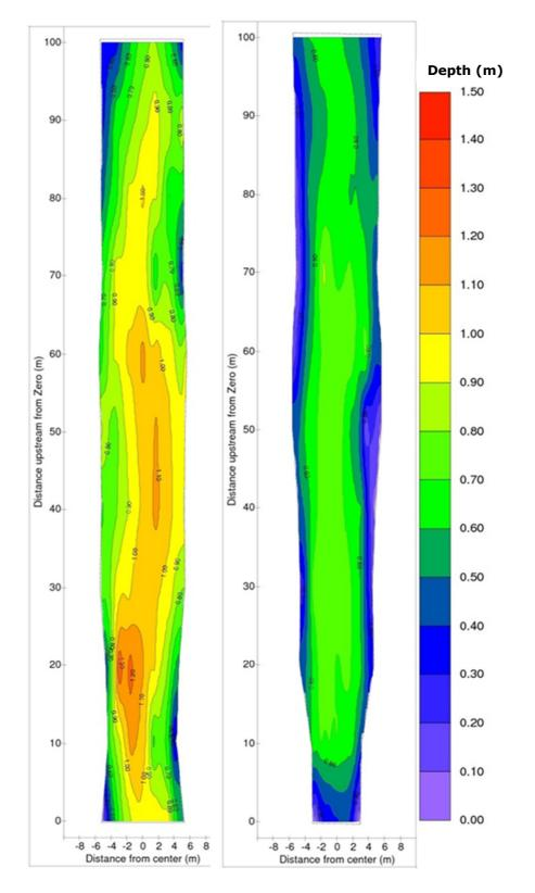
Figure 4.13. Depth (m) contour plots of the 100m upstream of Milltown Bridge pre (left – 2013) and post (right – 2015) removal of horseshoe weir and construction of alternating deflectors.
