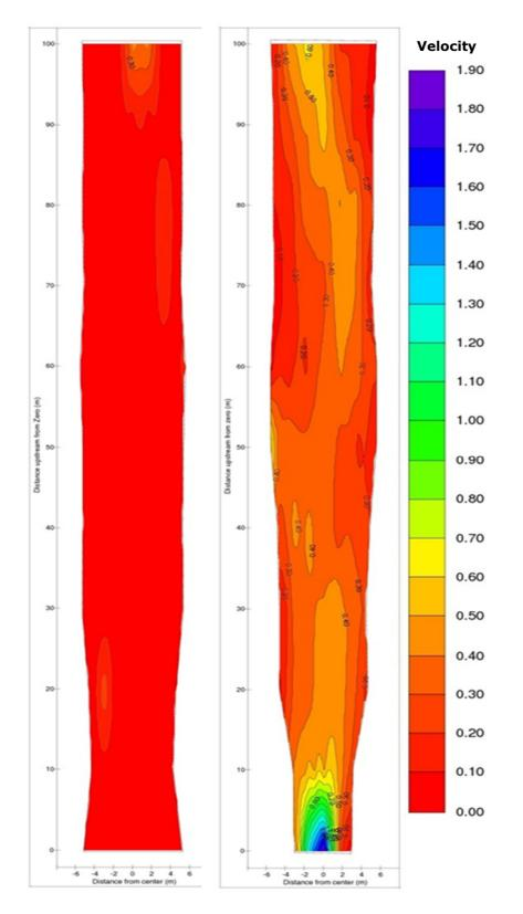
Figure 4.14. Velocity (m/sec) contour plots of the 100m upstream of Milltown Bridge pre (left – 2013) and post (right – 2015) removal of horseshoe weir and construction of alternating deflectors.
