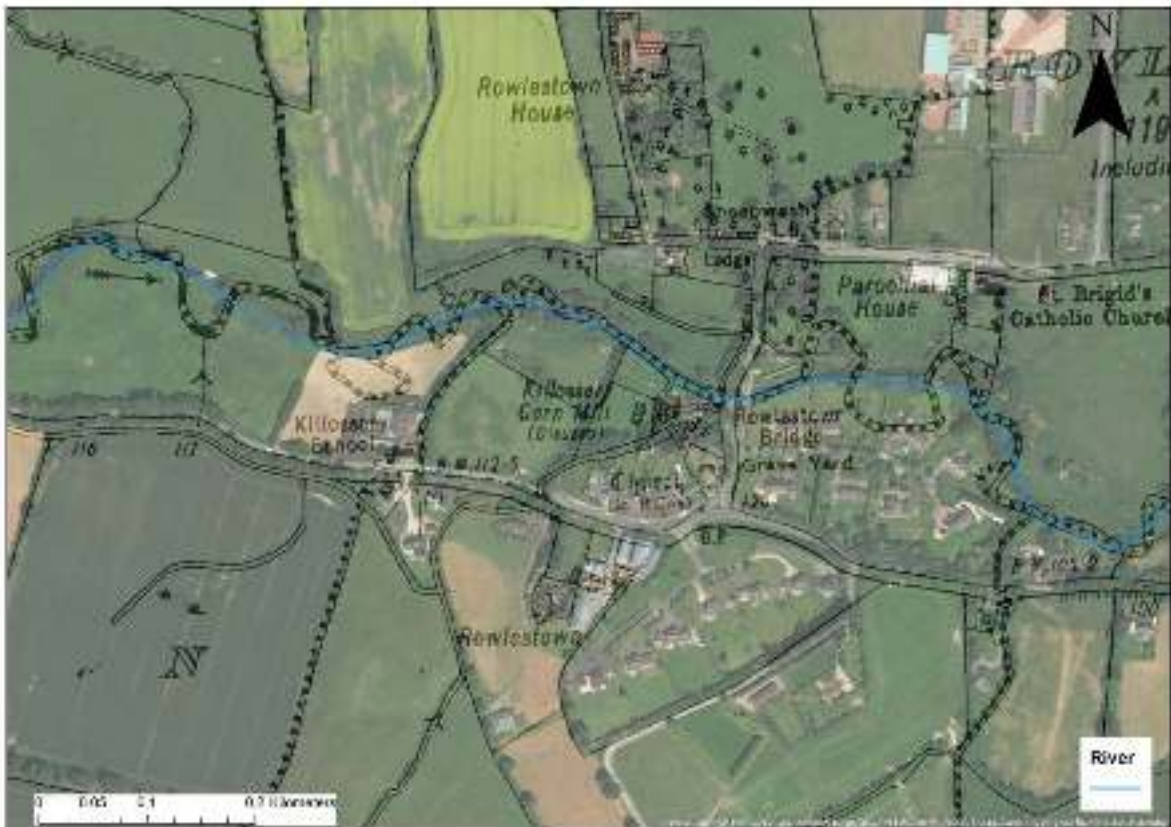
Figure 2.37. Historic maps over-lapping aerial imagery showing the extent of straightening in OPW channels in both Rural (Nenagh River) and Urban Areas (Broad Meadow River, Swords).
