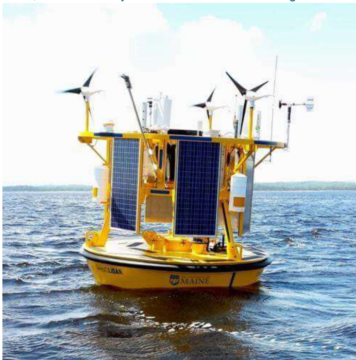
Figure A 9 Floating LiDAR buoy (Wind Power Engineering & Development, 2016)
