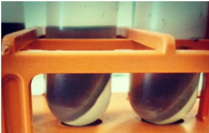
Figure 5 Extraction of total lipid using Chloroform and methanol
