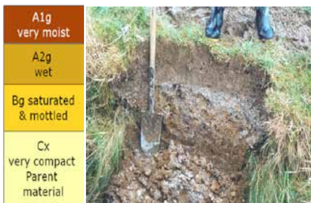
A very poorly-drained 'dauby' gley soil profile with a clay-rich topsoil approx. 30 cm deep, which overlies a saturated & mottled, blue-grey & red-brown subsoil. The subsoil overlies a very compact parent material derived from glacial till.
