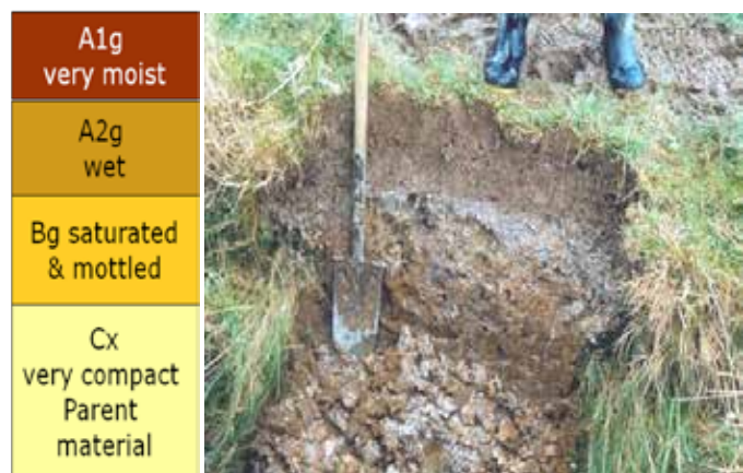
A very poorly-drained 'dauby' gley soil profile with a clay-rich topsoil approx. 30 cm deep, which overlies a saturated & mottled, blue-grey & red-brown subsoil. The subsoil overlies a very compact parent material derived from glacial fill.
