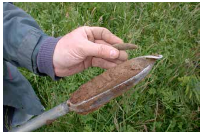
Figure 2 A topsoil core sample taken with a Dutch soil auger.
