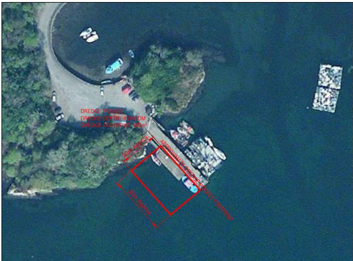
Figure 4. Glengarriff Pontoon approximate dredge footprint
