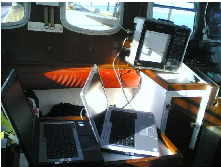
The ODOM Hydrotrac digital echosounder recorder set up onboard during survey.
