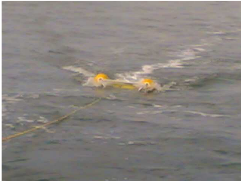
Towed catamaran with seismic source for C-boom subbottom profiling system
