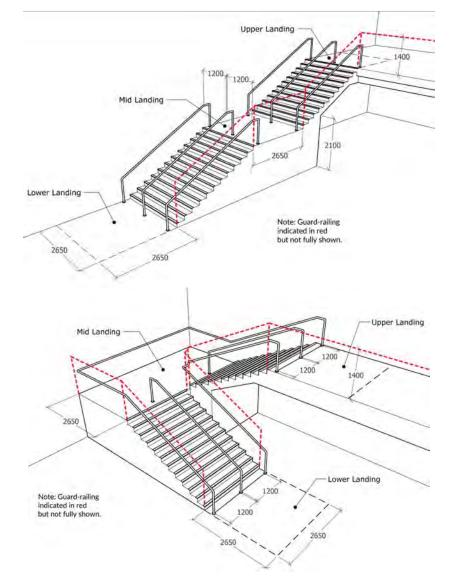
b. Fire escape stairs should have sufficient width to allow the safe escape of students, in compliance with the fire escape strategy and the approved Fire Safety Certificate. The flights and landing must be protected by guarding that have a minimum height of 1,400mm. The staircase must fully comply with the requirements of the current related Building Regulations.
