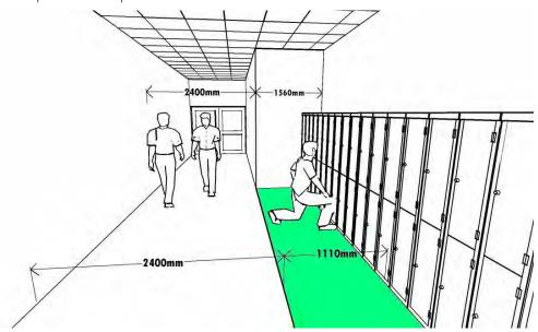
d. A lift shall not reduce the minimum width requirements for circulation within its vicinity. A landing turning area of 1.8 m x 1.8 m must be available at entrance doors to lifts.
