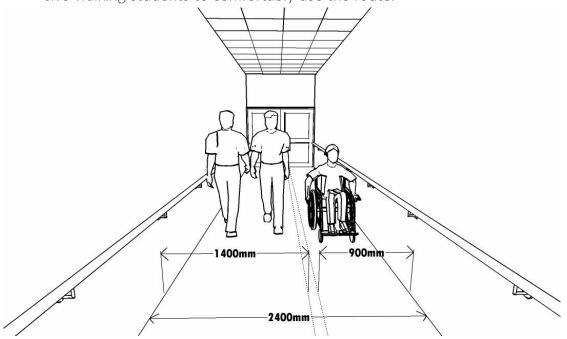
c. A minimum recess for lockers of 1.56m (as per diagram below) off circulation routes is required to ensure uninterrupted clear pathways, particularly in emergencies, and also for the safety of disabled or visually impaired. Access to lockers must not compromise Pupil Social Areas.
