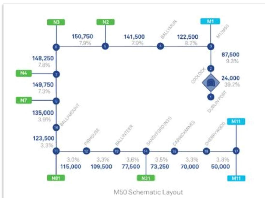
Figure 4: Annual Average Daily Traffic (% Heavy Goods Vehicles) on M50 in 2019 (Source TII)
