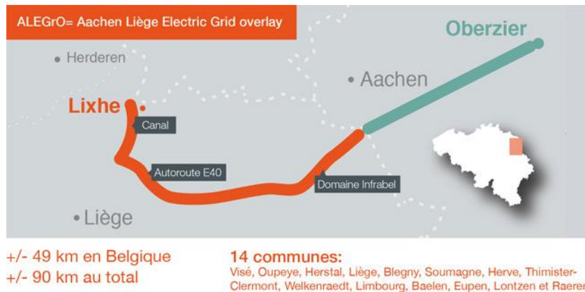
Figure 12: ALEGrO project: cable routing [29]
