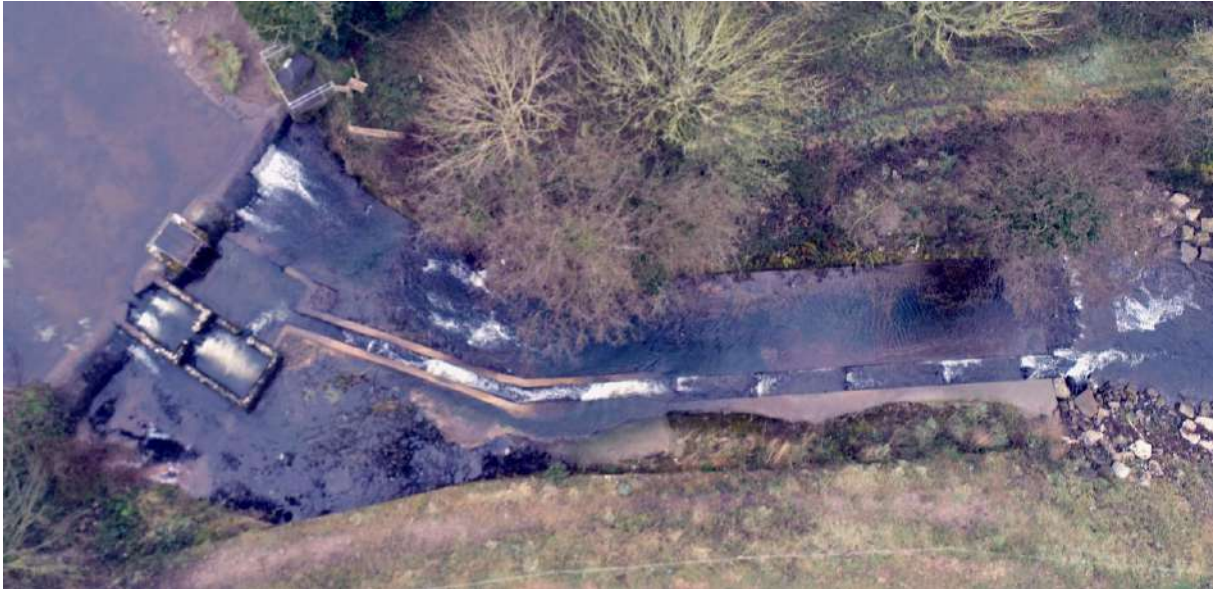
Figure 7.5 Drone image of the gravel trap on the Kilcormac Silver, Brosna catchment (ST6).
