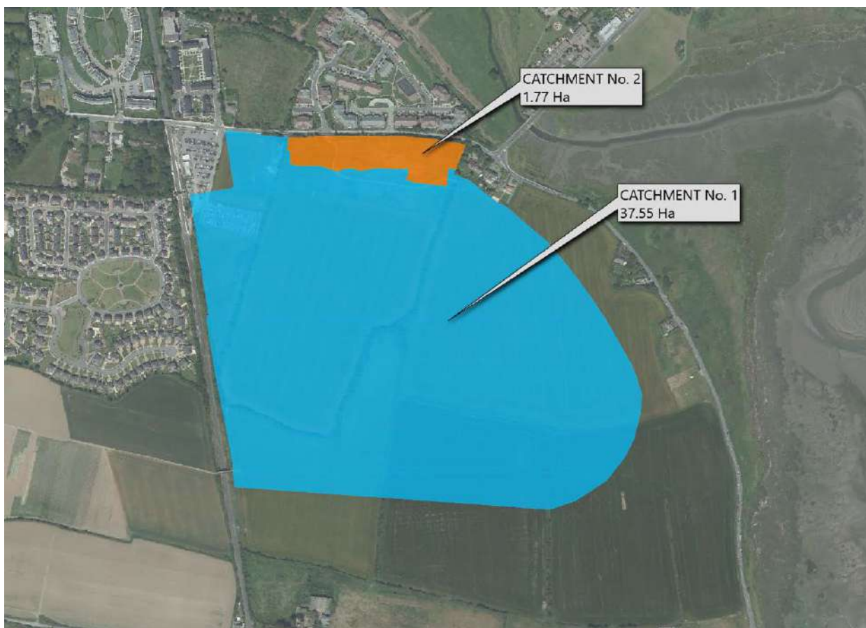
Figure 7 Surface water catchments for the Portmarnock South LAP lands. The area in blue is accommodated in the new regional wetland, to be delivered as part of Phase 1B. The area in orange is accommodated in a new detention basin, also to be delivered as part of Phase 1B.
