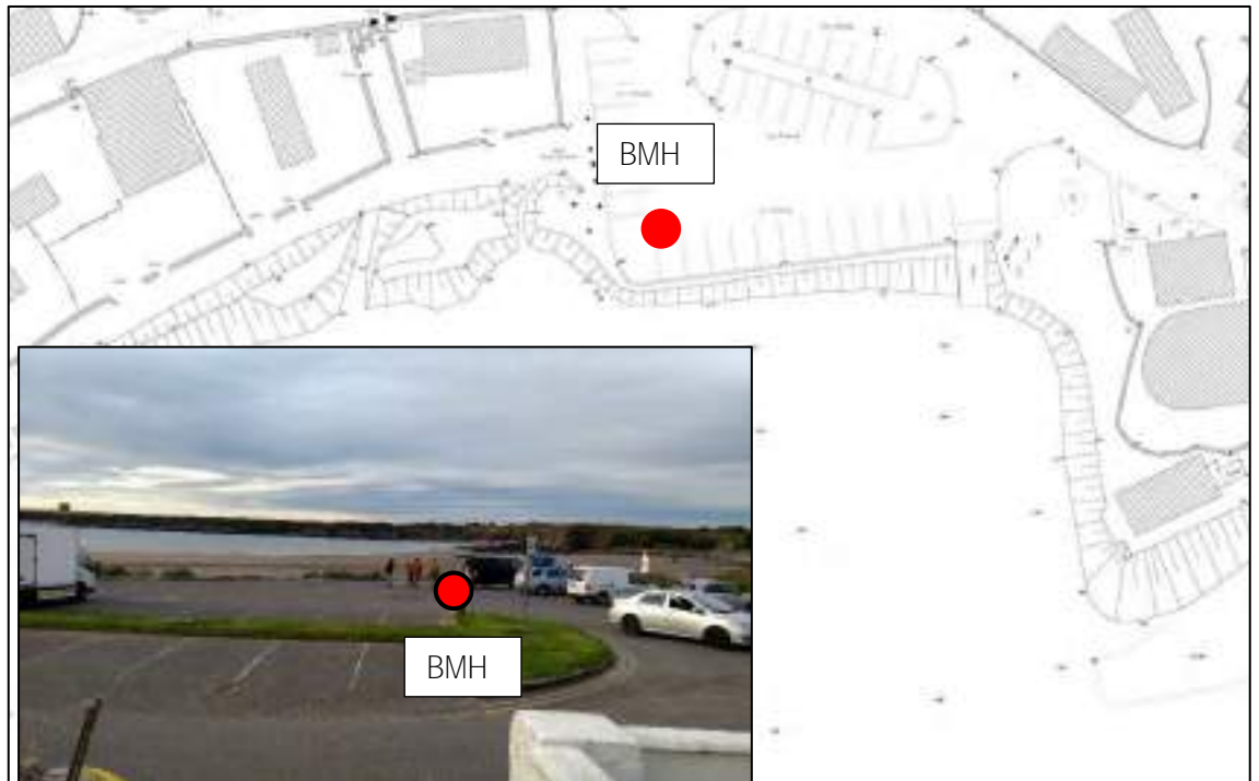
Figure 4.37: Land survey chart- illustrating the BMH position at the southwestern corner of the parking lot.
