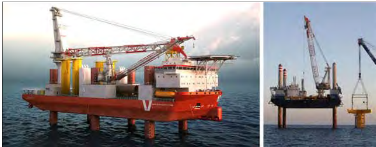
Figure 2.8 Typical Jack-Up Vessels used for foundation and turbine installation
