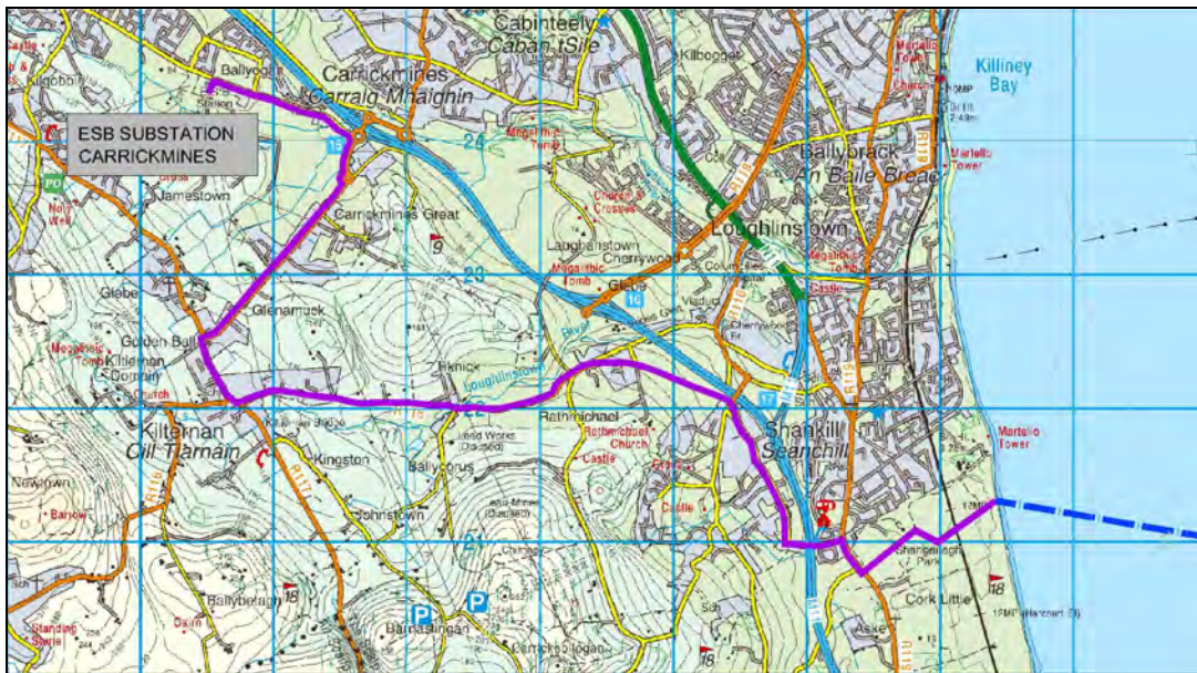
Figure 4.4 Export Cable Landfall and Indicative Onshore Cable Route (OSI License No. EN0034812)
