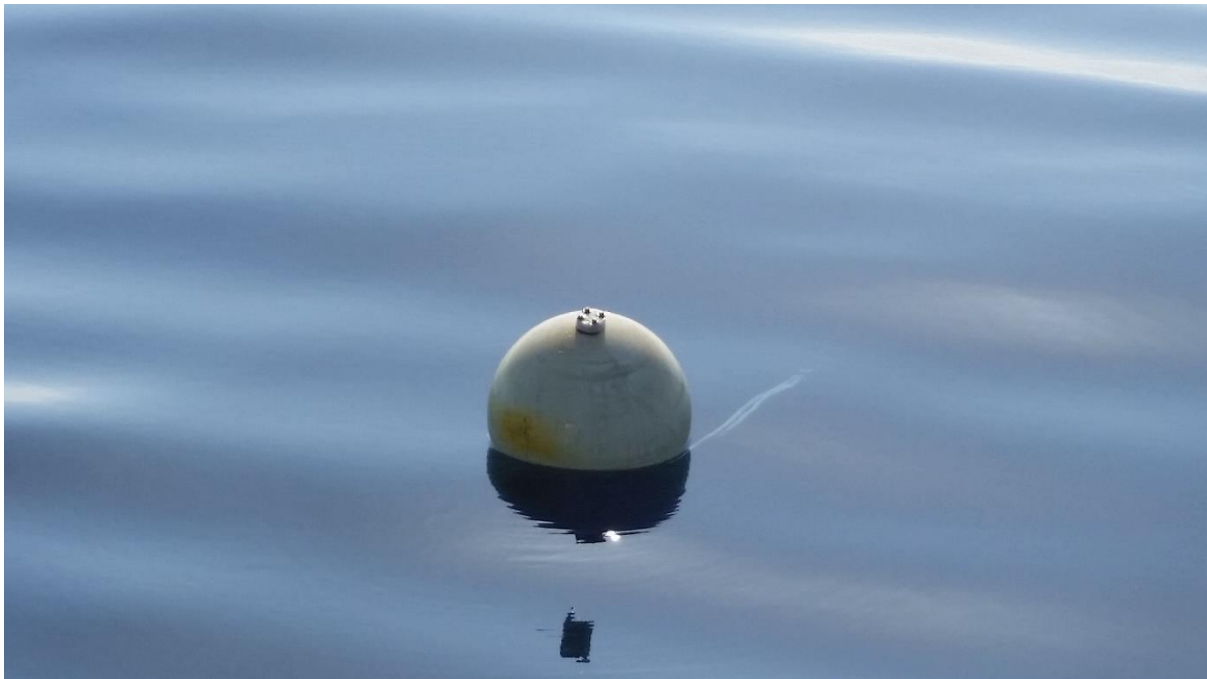
Figure 2: The recovery buoy after surfacing.
