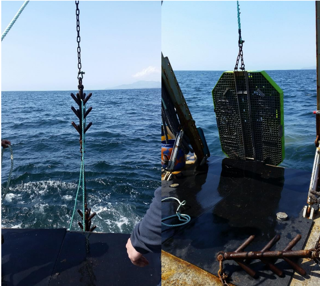
Figure 5: Left -The grapple hook caught with the grapple line. Right - The floating grapple line is winched into retrieve the ADCP frame.
