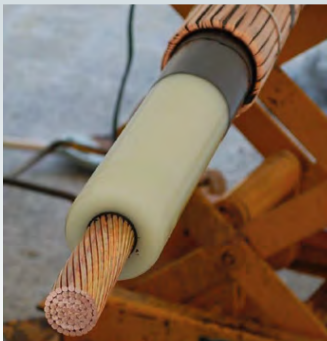
Example of a HV DC bi-pole cable featuring copper core, XLPE insulator, semiconducting screen and concentric copper return conductors
