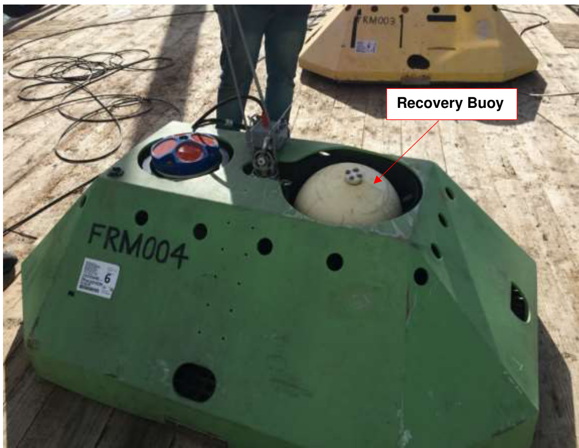
Figure 3: Acoustic Release Recovery Buoy.
