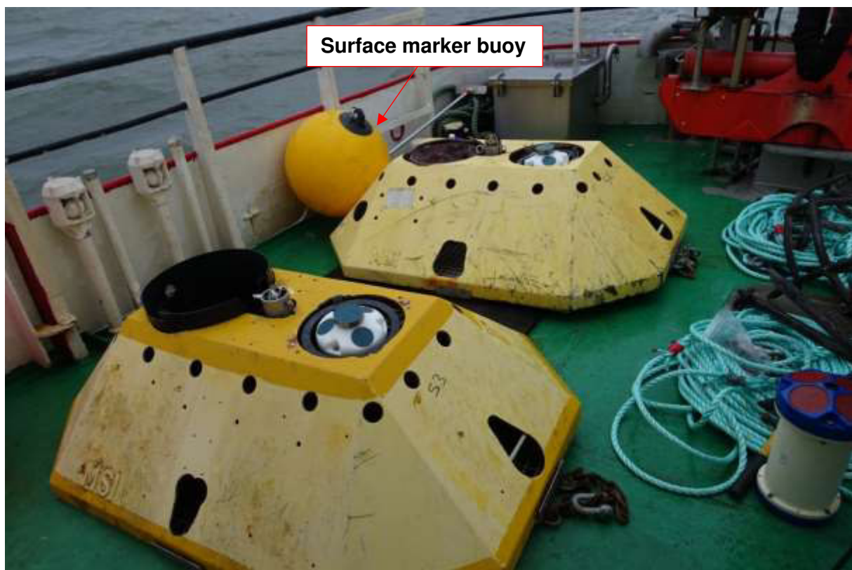
Figure 1: Yellow Surface Marker Buoy & ADCP Frames.
