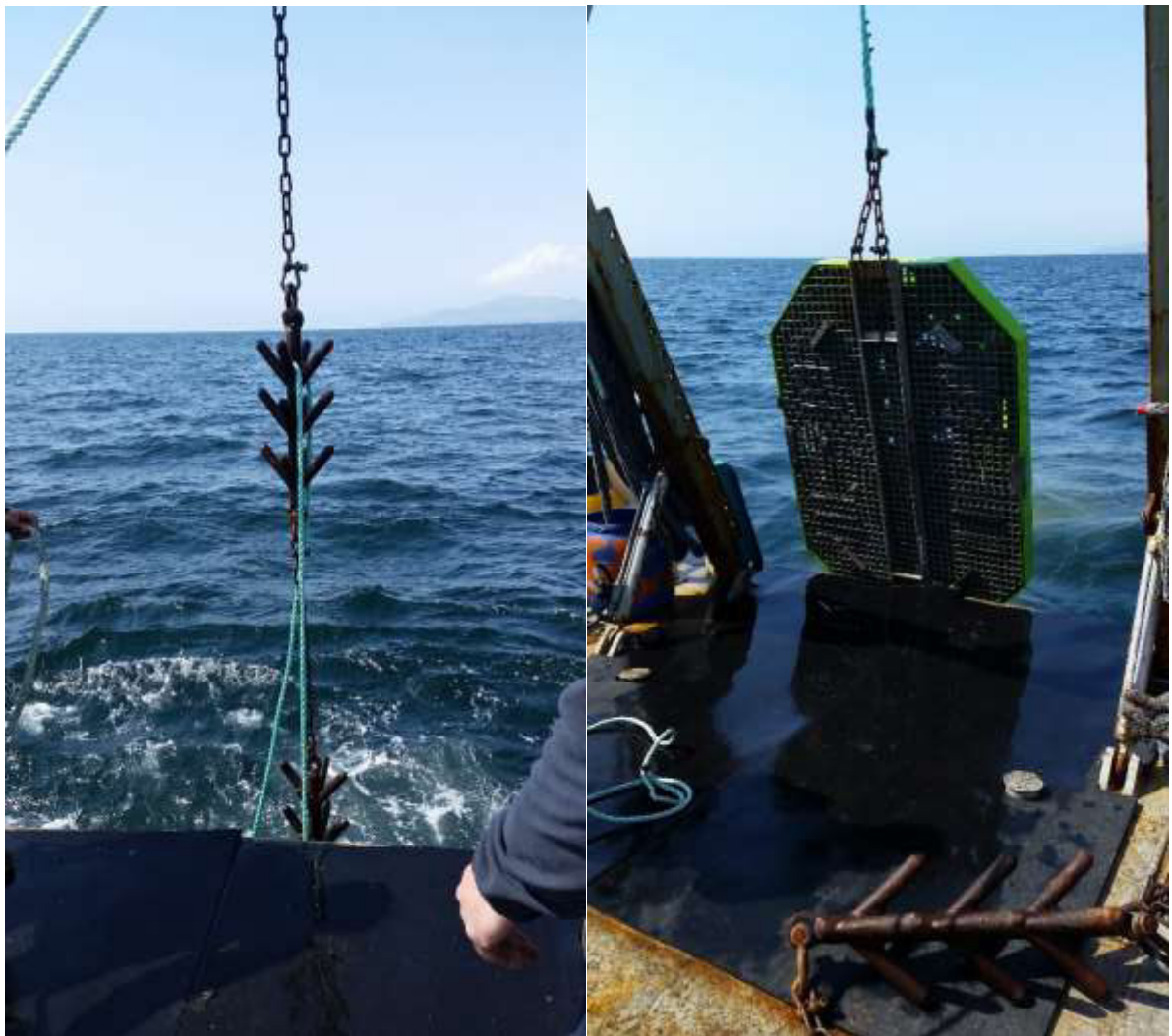
Figure 5: Left - The grapple hook caught with the grapple line.
