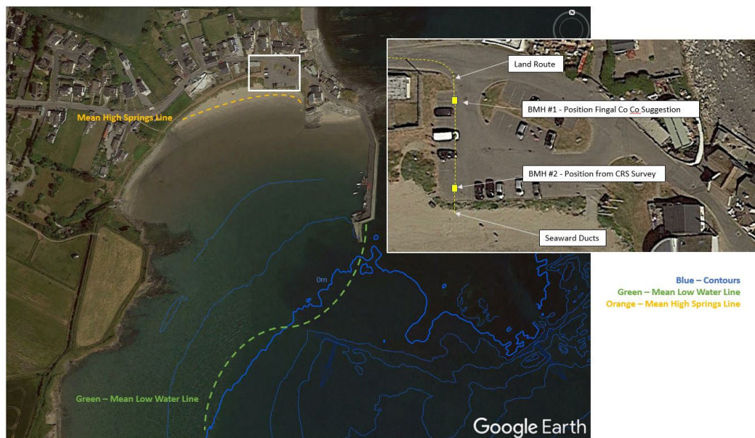
Figure 2-13 Overview image of Loughshinny landing site showing the location of the BMH in the beach car park, and the relative mean tide lines
