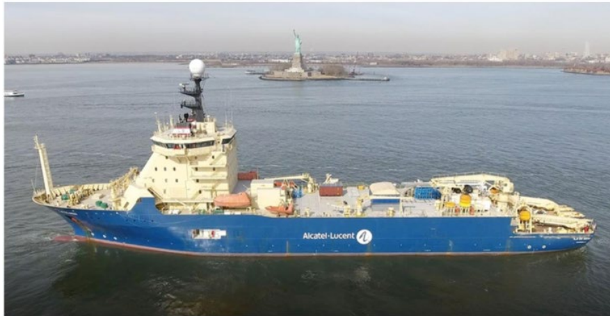
Figure 2-8 Cable lay vessel example
